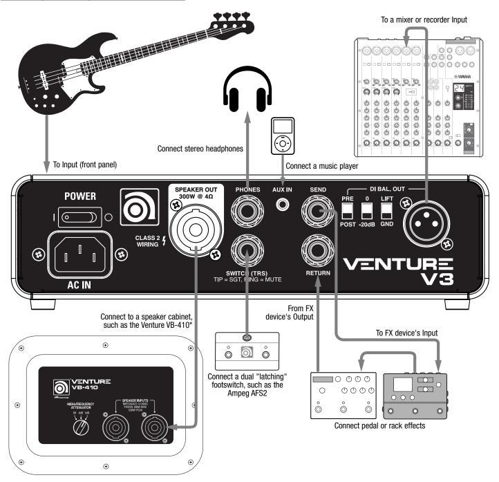
\*NOTE: Total impedance for all connected speaker cabinets should never be less than 4 Ohms. Always use speaker cabinets with the same nominal impedance when using more than one cabinet.
