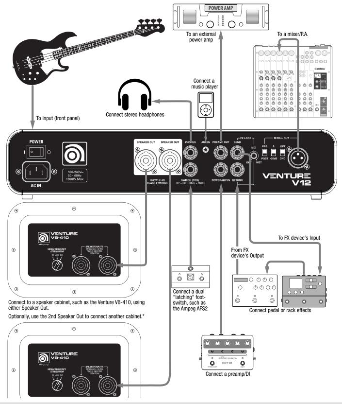
\*NOTE: Total impedance for all connected speaker cabinets should never be less than 4 Ohms. Always use speaker cabinets with the same nominal impedance when using more than one cabinet.
